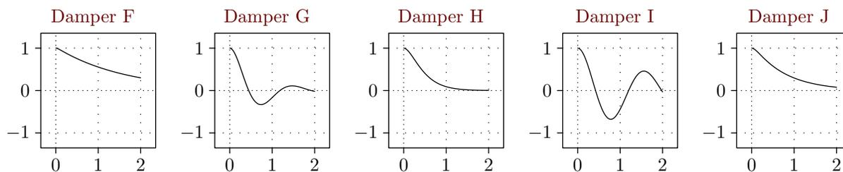
(a) For which damper is the system critically damped?
