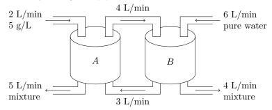
Write the differential equations and initial conditions that describe the amount of salt in each tank.
